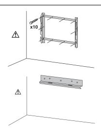
■ The Wall Mounting Unit should be mounted to a wall that can adequately hold the total weight of the plasma display and the Wall Mounting Unit over a long period of time and which can adequately withstand earthquakes, conceivable vibrations, and other external forces. Improper installation may cause the plasma display to fall down, resulting in physical injury.
